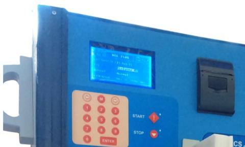
**DCS-*plus*** gives the user, documentation of dialyzer status with date and time stamp through an in-built thermal printer.
